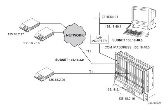
Figure F-2. Local Carrier with Remote Standalone
